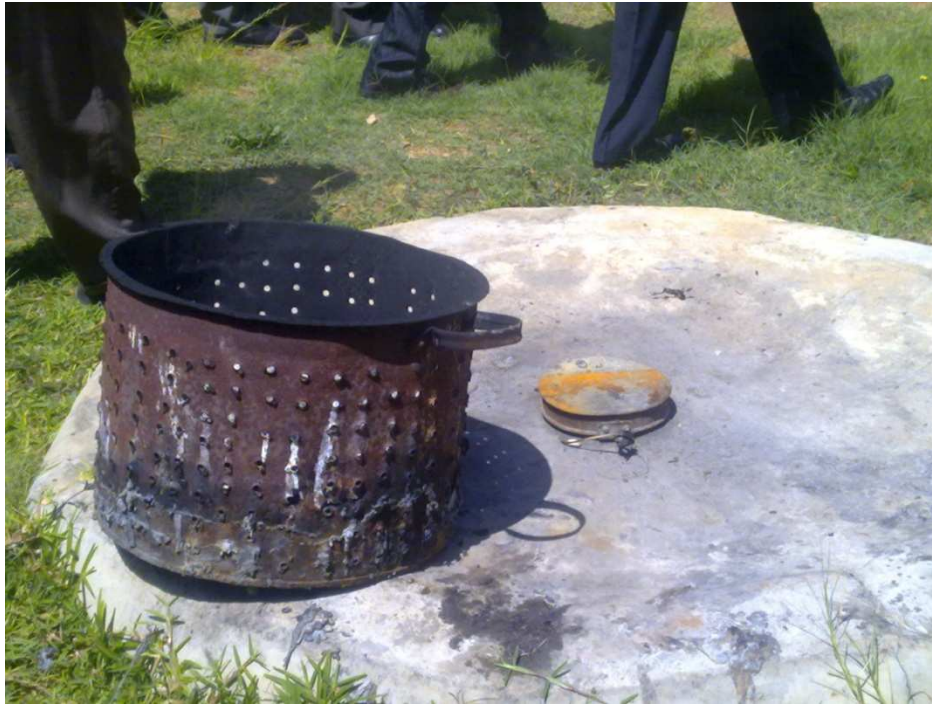
An improvised incinerator at Mansa Clinic
